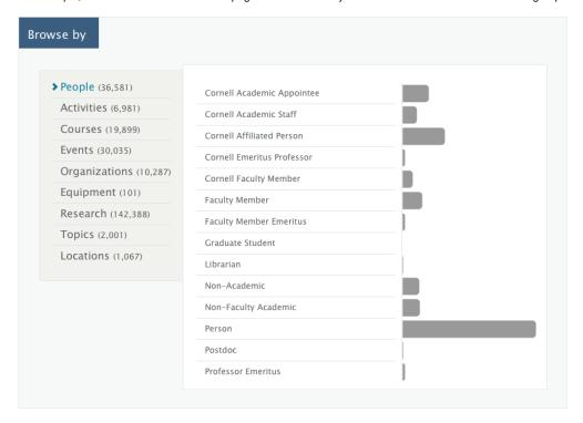
VIVO could produce this data by issuing a SPARQL query against its data model. However, this would take several seconds for a large site, and we do not want the user to wait that long to see the home page. To avoid this delay, the class group of each individual is stored in the Solr record for that individual. Solr can count these fields very quickly, so VIVO issues a Solr query against the index, and displays the results on the home page.
